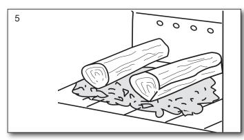
Now open the combustion air completely. If the stove and/or chimney cools down too much, it may be necessary to have the door ajar. The wood will then ignite within a very short time (Typically 1 to 3 minutes). Once the fuel is Ignited. Close the door and regulate the air back to operating air. When the fire is well established, you can now regulate the operating air to the desired combustion level.
