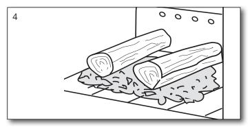
most towards the front of the stove. Place firewood equivalent to 1.6 kg on top of the embers in one layer, perpendicular to the chamber opening. See fig. 4.
